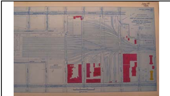
One of the biggest challenges during construction was keeping track of previous structures uncovered during the excavation. A special note on this map (dated June 1904) of existing conditions makes no claim that sub-surface features depicted are "even approximately correct." 7
